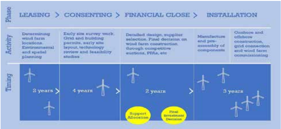
Figure 8: Offshore Wind Power Plant Development Stages 47
